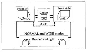
In a system without a center speaker: The test tone will be heard automatically from the front left and right speakers and the rear speakers alternately.
