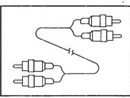
One RCA pin-type video cable, (if connecting a standard VCR), or
