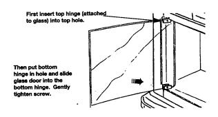
The glass door should open and close easily without rubbing on the stand. You can adjust the position of the glass door if necessary by slightly loosening the hinge screws, moving the door, and then retightening the screws.
