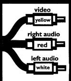
AUDIO/VIDEO CABLES, also called RCAtype cables, usually come in groups of three cables, each one with a connector that is color-coded according to its use: yellow for video; red for right audio; and white for left (or mono) audio.
