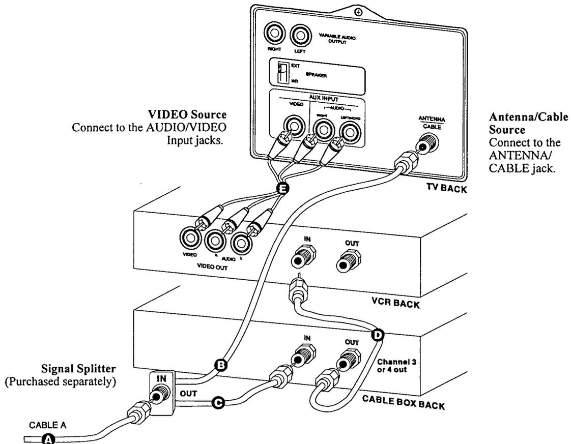
**Option 2: Cable-TV Connection Direct to TV & Cable Box to VCR.**
