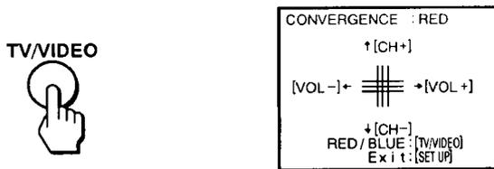
(3) Using CHANNEL+/- or VOLUME+/-, move the line until it converges with the center green line.
