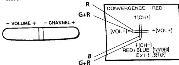
To move horizontal line up/down, press CHANNEL +/-.
