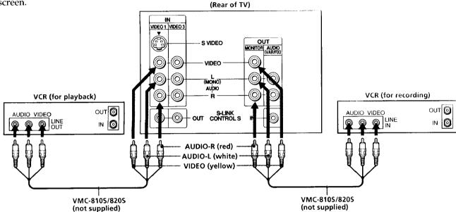
The above type of connection should only be used when you connect from the line input of one VCR, and from the line output of a second VCR.
