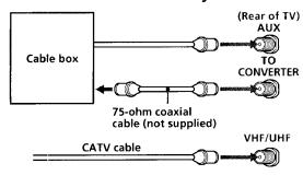
Pay cable TV systems use scrambled or encoded signals requiring a cable box\* in addition to the normal cable connection.
