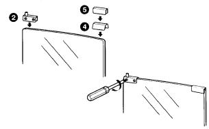
3 Push the top, glass door hinge into the top, right bushing and gently slide the glass door into the bottom hinge. Adjust the glass door until level, and tighten the hinge screws.
