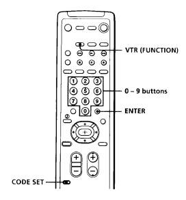
Press the CODE SET, VTR (FUNCTION), and 0 – 9 buttons to enter the manufacturer's code number (see the chart), then press ENTER. For example, to operate a Sony 8 mm VCR, press CODE SET, VTR (FUNCTION), 3, 0, 2, and ENTER.
