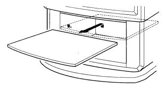
3 Insert shelf supports in the appropriate holes. Slide shelf in, align the shelf grooves with the shelf supports, and slide the shelf down.
