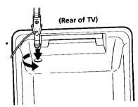
**2** Attach the antenna connector to the VHF/UHF terminal.
