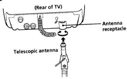
**2** Attach the antenna connector to the VHF/UHF terminal.
