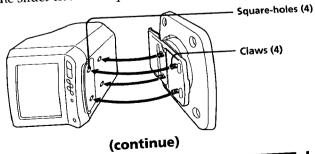
**3** ① Push the base in the direction of the arrow ① until the two rear claws on the slider touch the back of the square-holes on the bottom of the TV.
