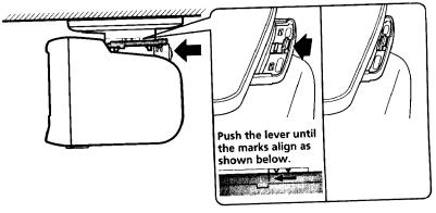
Make sure that the bracket and the TV are locked completely.
