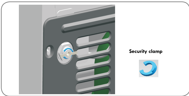
Step 1 ) Remove the security clamp.
