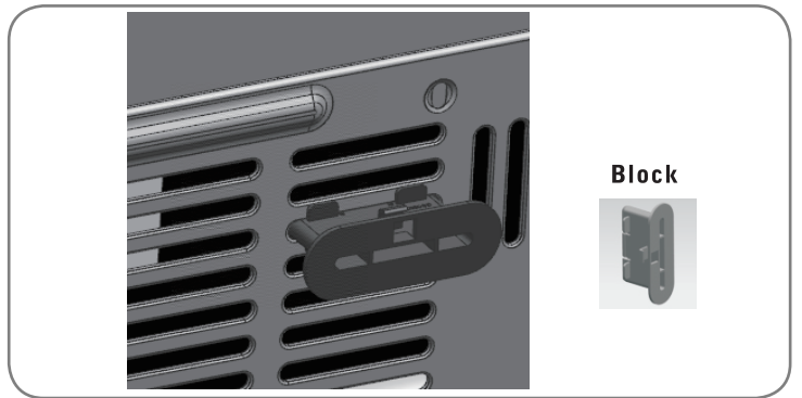
Step 5 ) Install the block.
