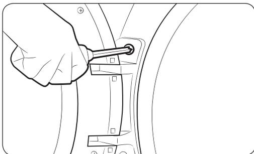
10. Place the door on the other side, and then reattach it to the dryer.
