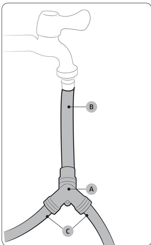
1. Close the cold water tap. If you have a washer cold water hose attached to the cold water faucet, unscrew and remove the hose. Then, connect the **short hose (B)** to the cold water tap. Turn the coupling by hand until it is tight.
