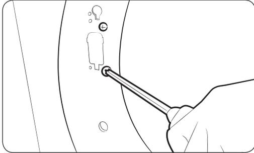
7. Re-insert the two screws that held the lever holder into the same screw holes, and then tighten.
