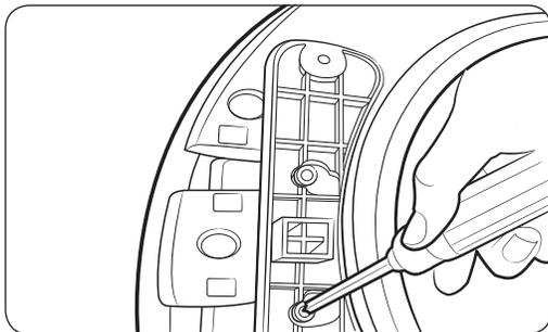
8. Remove the single screw from the back of the door hinge.
