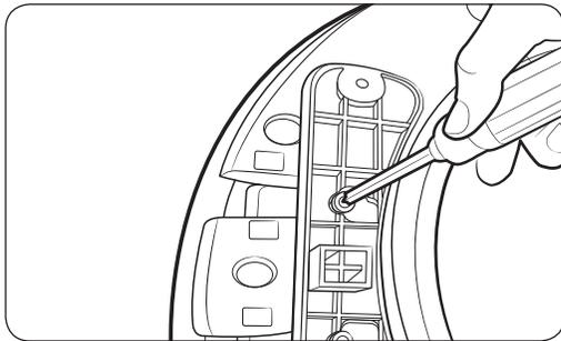
9. Insert the screw you just removed into the other screw hole on the back of the door hinge, and then tighten.
