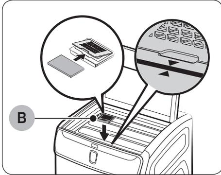
3. Insert a folded dryer sheet in **dryer-sheet case (B)**, and then put the case at the top center of the rack. Make sure the dryer-sheet case faces against the triangle mark on the Delicate Dryer because only the arrow area has the built-in magnet to secure the filter.
