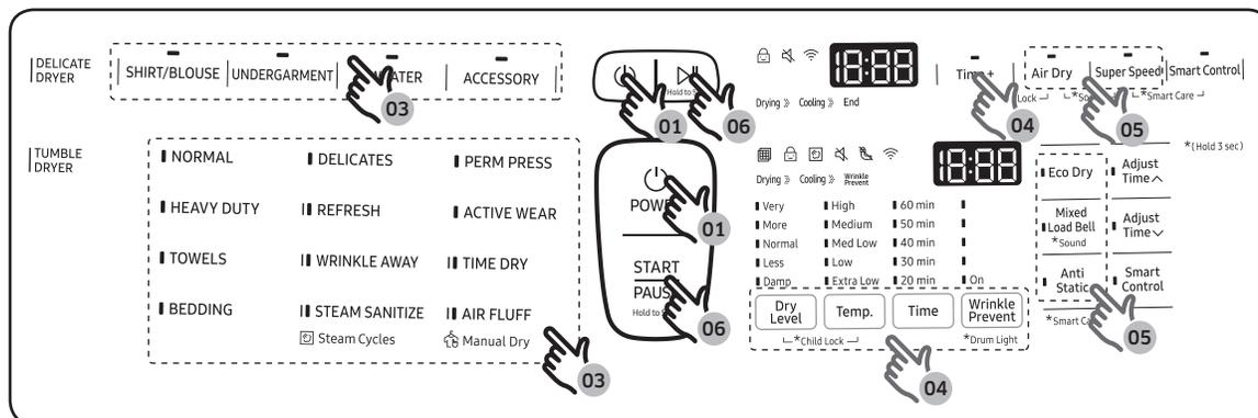
1. Press **POWER** on the control panel of a desired dryer (Delicate, Tumble) to turn the dryer on.
