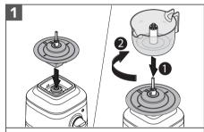
Place the Gear Assembly on Base. Place the Juice Container on the Gear Assembly and twist clockwise to lock in place.
