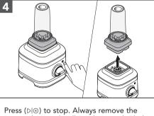
Personal Jar or Small Batch Jar with Blade Assembly from the Base.
