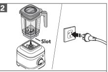
Place and align the Jar with the Slot to fit inside the jar pad, facing Jar handle towards Control Dial. Plug the Blender into an earthed outlet.
