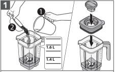
Add ingredients into Jar (max. 1.6 L or 1.4 L for Glass Jar). Secure the Lid and Lid Centre Cap.
