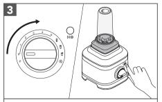
Turn from (**O**) to desired speed or preset recipe programme. Press  $(\triangleright | \otimes)$  to start. See "Blender Function Guide" for more details.
