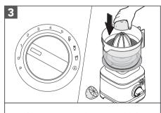
Turn from (**O**) to speed **1** or **2**. Hold down the halved citrus fruit on the Reamer. Press  $(\triangleright \otimes)$  to start.
