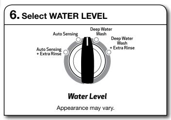
Set the Water Level knob to the Auto Sensing setting and the washer will fill to a level that ensures the load engages the agitator. From this point, the electronic control will sense the load and determine if additional water is needed. Select Extra Rinse for enhanced rinsing performance.
