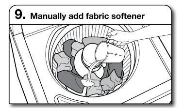
During the final rinse, wait until the washer has completed filling, then press START/STOP/PAUSE/UNLOCK LID to pause the washer. Lift the lid and add the measured recommended amount of liquid fabric softener. Do not use more than the recommended amount. Close the lid and press START/STOP/PAUSE/UNLOCK LID again to start the washer.
