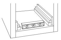
• Use the leveling legs to adjust level front to back and side to side.
