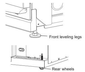
• Place a level inside the compactor on the floor of the cabinet.
