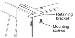
• If the brackets cannot be attached to the underside of the countertop, attach mounting clips to the bracket. Fasten the compactor to the cabinet front with mounting screws through the mounting clips.
