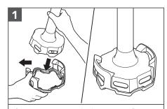
If using a Pan Guard, place it on a flat surface. To insert the Pan Guard, angle the Blending Arm to one side of the mounting clip. Then, gently pull the other mounting clip outward and push down the Blending Arm. Ensure the Mounting Clips are secured into place.
