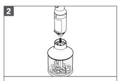
Align the Chopper Attachment with the Motor Body and press together. Do not twist the Motor Body into place.
