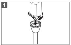
In order to charge the battery, twist to unlock and remove the Blending Arm.
