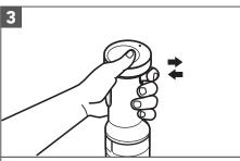
Press the Variable Speed Controller and Palm Switch at the same time to start.
