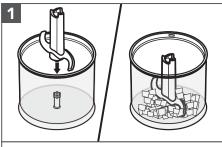
Insert the Chopper blade into Chopper bowl. Add ingredients into the Bowl. For best results, cut the food items into 3/4" (2 cm) pieces.
