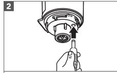
Plug in the Charger Adapter Pin into the Charging Port.
