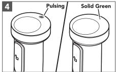
The Battery Status Indicator pulses when it charges. It will be fully charged in 2 hours and the Battery Status Indicator turns solid green.
