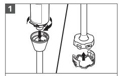
Remove the Blending Arm, Pan Guard, or Whisk accessory before cleaning.
