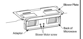
**9** Secure the blower plate to the microwave with screw.
