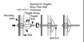
Place the mounting plate against the wall and insert the toggle wings into the holes in the wall to mount the plate.
