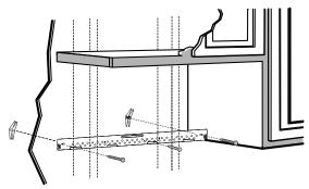
Attach the plate to the wall using toggle bolt. At least one wood screw must be used to attach the plate to a wall stud.
