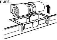
Roll the blower unit 90° so that fan blade openings are facing out the up of the microwave.
