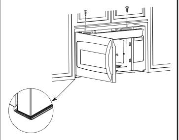
**A 5.7** Close the microwave door Plug in microwave oven or reconnect power.
