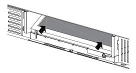
Reinstall the vent by sliding the bottom of the vent into place. Push the vent top into position and slide right into place. Replace the two vent mounting screws located on top of the microwave using a #1 Phillips screwdriver.
