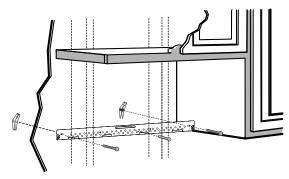
Attach the plate to the wall using toggle bolts At least one wood screw Inust be used to attach the plate to a wall stud.
