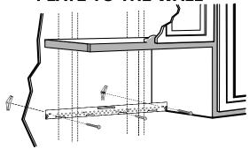
Attach the plate to the wall using toggle bolts. At least one wood screw must be used to attach the plate to wall stud.
