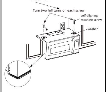
Tighten the outer two screws to the top of the microwave oven. (While tightening screws, hold the microwave oven in place against the wall and the top cabinet.)
