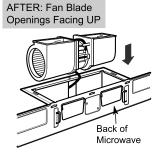
**CAUTION:** Do not pull or stretch the blower unit wiring. Making sure the wires are not pinched.
