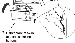
a Insert a self-aligning screw through top center cabinet hole. Temporarily secure the oven by turning the screw at least two full turns after the threads have engaged. (It will be completely tightened later.) Be sure to keep power cord tight. Be careful not to pinch the cord, especially when mounting flush to bottom of cabinet.
