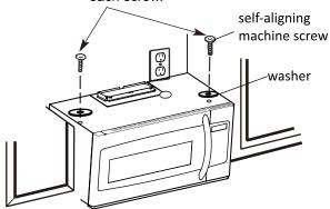
Tighten the outer two screws to top of the microwave oven. (While tightening screws, hold the microwave oven in place against the wall and the top cabinet.)
