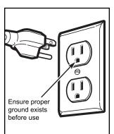
The power cord of this appliance is equipped with a three-prong (grounding) plug which mates with a standard three-pron (grounding) wall receptacle to minimize the possibility of electric shock hazard from this appliance.
