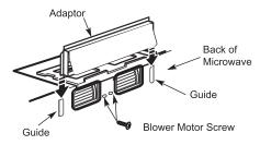
Push in securely until it is in the lower Blower Motor screw Take care to assure that the damper hinge is installed so that it is at the top and that the damper swings freely. 8 Secure the blower motor unit to the microwave with screw as before.
