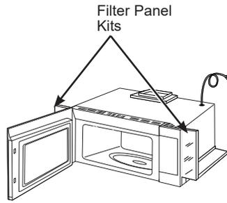
When replacing a 36" range hood, filler panel kits fill in the additional width to provide a custom built-in appearance.
