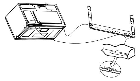
**Step. 2**Lift the microwave oven and tilt it forward.
