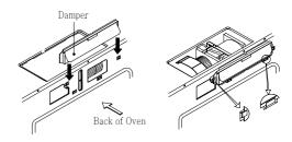
After adjust the damper, reinstall the blower motor cover with the screw  $(\widehat{1})$ .
