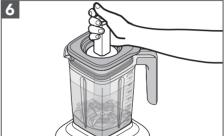
Tamper accessory: Remove the Lid Centre Cap only. Stir or press contents down towards the blade. Then, place the Lid Centre cap back before resuming blending.
