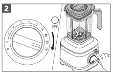
Turn from ( $\mathbf{O}$ ) to ( $\mathfrak{T}$ ). Press ( $\triangleright$ ( $\otimes$ ) to start. When cycle ends, remove the Jar and empty contents and rinse with warm water and dry thoroughly.
