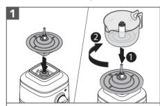
Place the Gear Assembly on Base. Place the Juice Container on the Gear Assembly and twist clockwise to lock in place.
