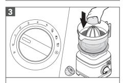
Turn from (O) to speed 1 or 2. Hold down the halved citrus fruit on the Reamer. Press  $(\triangleright | \otimes)$  to start.
