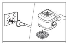
Unplug the Blender before cleaning. Wipe clean the Base, Power Cord and the Gear Assembly of the Citrus Press with a warm, damp cloth and dry with a soft cloth.
