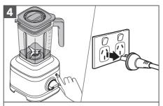
When finished, press ( $\triangleright | \odot$ ) to stop. Unplug before removing the Blender Jar.
