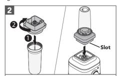
Secure the Blade Assembly on the Jar and rotate it clockwise until it is tight.
