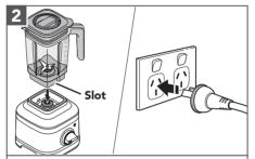
Place and align the Jar with the Slot to fit inside the jar pad, facing Jar handle towards Control Dial.
