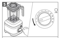
**Pulse mode:** Press ( $\triangleright$ | $\otimes$ ). Turn and hold the Control Dial from (**O**) to (**P**) as per desired interval of time.
