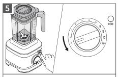
**Pulse mode:** Press  $(D| \otimes)$ . Turn and hold the Control Dial from  $(\mathbf{O})$  to  $(\mathbf{P})$  as per desired interval of time. When finished, release the Dial to STOP.
