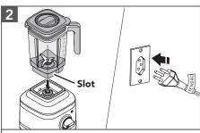
Place and align the Jar with the Slot to fit inside the jar pad, facing Jar handle towards Control Dial. Plug the Blender into earthed outlet.
