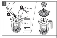
Add ingredients into Jar (max. 1.6 L or max. 1.4 L for Glass Jar). Secure the Lid and Lid Center Cap.
