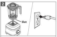
Place and align the Jar with the Slot to fit inside the jar pad, facing Jar handle towards Control Dial. Plug the Blender into a grounded 3 prong outlet.
