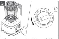
**Pulse mode:** Press  $(D| \otimes)$ . Turn and hold the Control Dial from  $(\mathbf{O})$  to  $(\mathbf{P})$  as per desired interval of time. When finished, release the Dial to stop.
