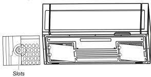
4. Put the grease filter back to the bottom plate.
