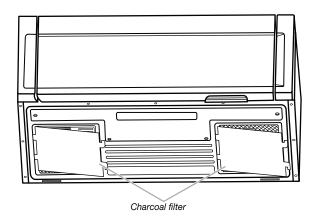
Replace a new charcoal filter and reattach it back to the bottom plate, and make sure both left and right sides insert into the bottom plate slots.
