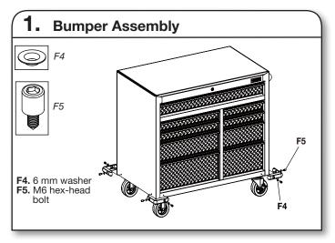
Using 6 mm hex head bolts (F5) (8) and 6 mm washers (F4) (8), fasten a bumper to each corner of the cabinet. Completely tighten all the fasteners.
