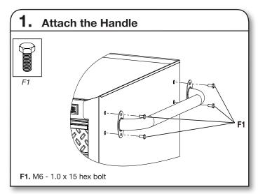
Position the handle over the threaded inserts on the side of the cabinet. Attach handle with M6-1.00 x 15 Hex bolts (F1) (4) and tighten with 10 mm wrench (provided).
