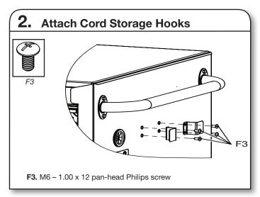
Position the cord storage hooks over the threaded inserts on handle side of the cabinet. Using M6-1.00 x 12 pan-head Philips screws (F3) (4) attach the hooks facing opposite of each other. Tighten the screws with a Philips screwdriver.
