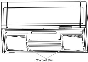
3. Replace a new charcoal filter and reattach it back to the bottom plate, and make sure both left and right sides insert to the bottom plate slots.
