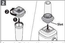
Secure the Blade Assembly on the Personal Jar and rotate it clockwise until it is tight. Place it on the Blender Base.
