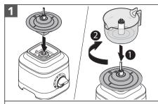
Place the Gear Assembly on the base. Then, place the Juice Container on the Gear Assembly and twist clockwise to lock in place.
