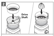
Place the Pulp Basket and then the Reamer into the Juice Container by aligning them with the Drive Shaft.
