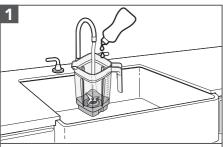
Empty the Jar. Fill half of the Jar with warm water and add 1 or 2 drops of dish-washing liquid.
