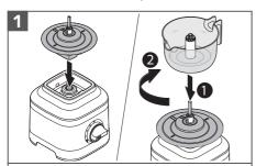
Place the Gear Assembly on the base. Then, place the Juice Container on the Gear Assembly and twist clockwise to lock in place.
