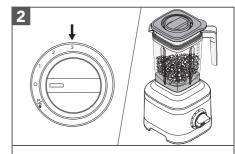
Run the Blender for 15-20 seconds on speed 3.
