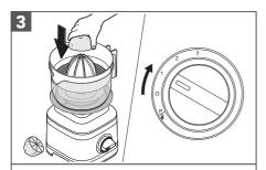
Hold down the halved citrus fruit on the Reamer. Turn the Control Dial from (**O**) to speed (**1**) to start juicing.
