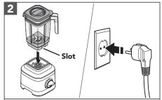
Place the Blender Jar on the base by aligning with the Slot to fit inside the jar pad, so that the handle of the Jar will be towards the Control Dial.
