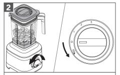
Turn and hold the Control Dial from ( $\mathbf{O}$ ) to ( $\mathbf{\mathcal{Q}}$ ) as per desired interval of time. When finished, release the Control Dial to stop the Blender.
