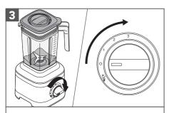
Turn the Control Dial from  $(\mathbf{O})$  to desired speed for constant operation.
