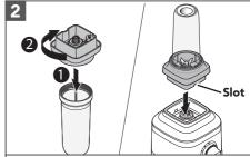
Secure the Blade Assembly on the Personal Jar and rotate it clockwise until it is tight. Place it on the Blender Base.
