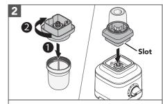
Secure the Blade Assembly on Small Batch Jar and rotate it clockwise until it is tight. Place it on the Blender base.
