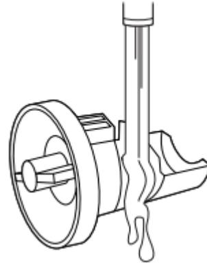
5. Reinsert the drain pump filter by turning it clockwise. Make sure to turn it in as far as it will go, with the filter handle remaining as close as possible to the vertical position.
