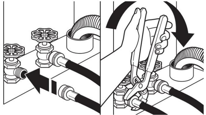
**IMPORTANT:** Do not overtighten or use tape or sealants on valve when attaching to faucets or washer. Damage can result.
