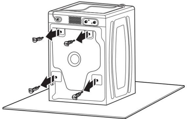
Loosen bolts with a 5/8" (16 mm) wrench. Slide each bolt and spacer to center of hole. Pull bolts and plastic spacers from back of washer. Discard bolts and spacers.
