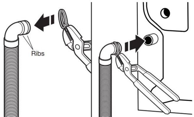
If clamp is not already in place on elbow end of drain hose, squeeze clamp with pliers and slide it over end of hose, centering it between the ribs, as shown. Squeeze clamp with pliers and slide elbow end of drain hose onto drain port and secure with clamp.
