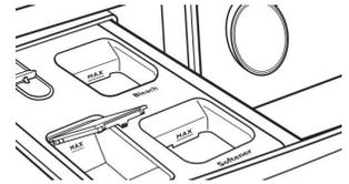
**NOTE:** Do not add single-dose laundry packets, Oxi-type boosters, color-safe bleach, or fabric softener crystals to dispensers. They will not dispense correctly. The Optimal Dispense Drawer cannot be disabled.
