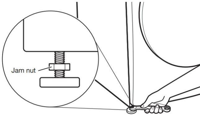
If washer is not level, use a 9/16" (14.3 mm) open-end or adjustable wrench to turn jam nuts clockwise on feet until they are about 1/2" (13 mm) from the washer cabinet. Then turn the leveling foot clockwise to lower the washer or counterclockwise to raise the washer. Do not exceed 2" (50 mm) from bottom of foot to bottom of cabinet. Recheck levelness of washer and that all four feet are firmly in contact with the floor. Repeat as needed.
