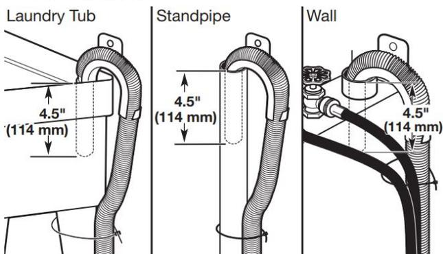
Secure drain hose to laundry tub leg, drain standpipe, or inlet hoses for wall standpipe with cable tie or beaded tie strap.
