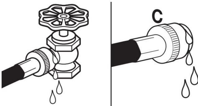
Slowly turn on water faucets to check for leaks. A small amount of water may enter washer. It will drain later.
