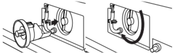
6. Replace and close the dispenser drawer. Make sure to insert both rails simultaneously when replacing the drawer. You will hear a clicking sound that indicates the rails have engaged. To ensure proper placement of the drawer, pull out fully. The drawer should be fully engaged and the rails locked in place. Make sure the drain hose is secured in the hose clip and tucked underneath the cutout.
