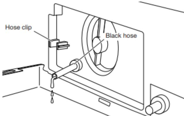
3. Lay a cotton cloth beneath the drain pump filter to absorb any water still in it. Then remove the drain pump filter by turning it counterclockwise.
