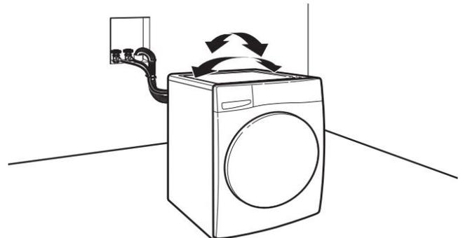
Grip washer from top and rock back and forth, making sure all four feet are firmly on floor. Repeat, rocking washer from side to side. If washer rocks, go to step 15 and adjust leveling feet. If all four feet are in firm contact with floor, go to step 16.
