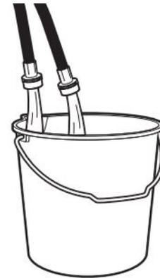
Run water for a few seconds through hoses into a laundry tub, drainpipe, or bucket to prevent clogs. Water should run until clear.
