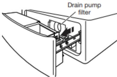
With your finger, push down on tab on right side of drawer, and up on tab on left side of drawer.
