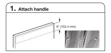
Install the custom hardware handle(s) on the front of the wooden panel inside dotted line.
