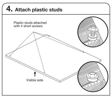
Attach the 4 plastic studs to the wooden panel using the four 5/16" hex-head (short) screws provided.
