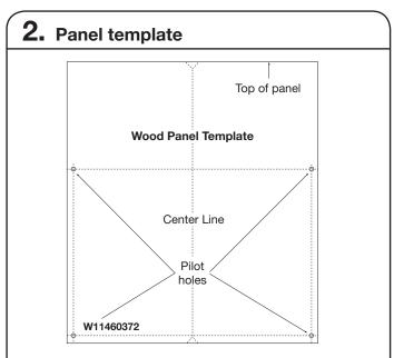
Using the template provided, attach it to the backside of the custom panel with tape. Make sure that the center of the template is aligned with the center of the wooden panel and top of the template is aligned to the top face of the wooden panel.
