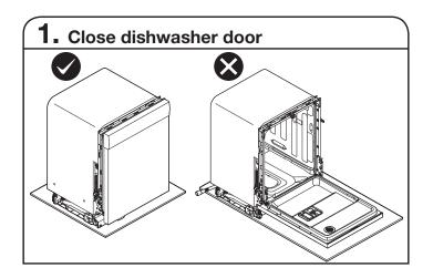
Make sure that the dishwasher door is closed at all times while hinge spring tension is being adjusted. Adjusting the hinge spring tension while the door is partially or fully open can cause damage to the hinge.
