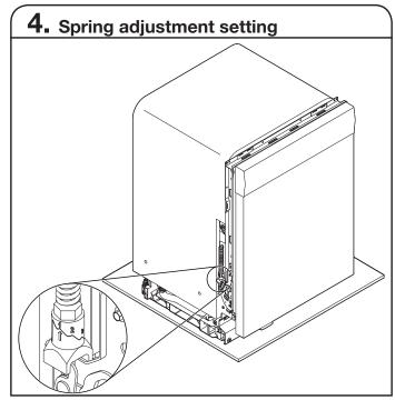
Each of the two hinges (right side and left side) have 3 different spring tension adjustments. All dishwasher models leave the factory with the hinges set in the lowest spring tension setting. This setting is suitable for lighter door panels. Heavier door panels will require adjustment of the hinge spring tension to prevent the door from falling open when its unlatched.
