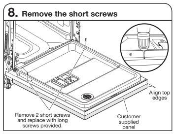
Remove the short screws (4<sup>th</sup> from top) on either side of the inner door panel. Use tape to mark a 3/32" drill bit to gauge the hole depth of approximately 1½" (38 mm). Drill 2 pilot holes using the door liner hole as a guide into the panel. Install the 2 remaining long screws.
