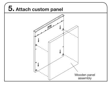
Align the studs on the custom wood panel to the keyhole slots on the door assembly. Ensure that all 4 plastic studs are engaged in the keyhole slots. Slide wood panel down until the top surface of the wooden panel is flush with the top of the door.
