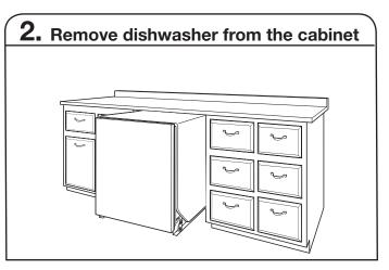
The dishwasher should be partially or fully removed from under the cabinet to grant access to the hinge spring tension adjustment mechanism.
