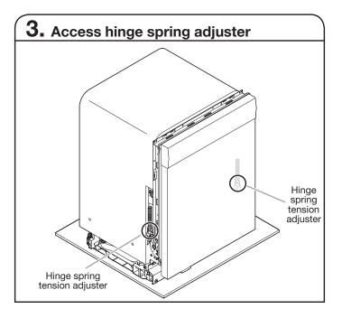
With the dishwasher partially or fully removed from the cabinet, the hinge spring tension adjusters can be accessed at the front sides of the dishwasher.
