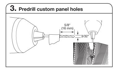
**NOTE:** Do not drill deeper then 5/8" (16 mm) to keep from drilling through panel. Pilot hole depths given are for 3/4" (19 mm) thick panel.
