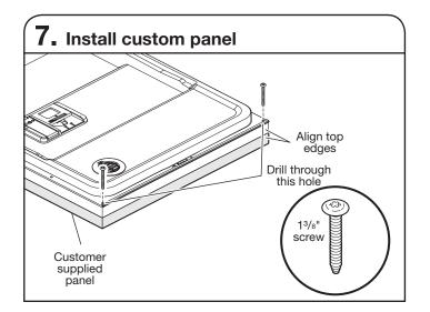
Using a Torx T15 screwdriver, install two #8 x 13/8" (long) screws in top corners to secure custom wood panel in place.
