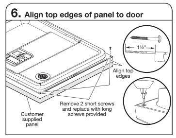
Open the door and align top edges. Use tape to mark a 3/32" drill bit to gauge the hole depth of approximately  $1\frac{1}{2}$ " (38 mm). Drill pilot holes into the top corners of the door, using hole in liner as a guide.
