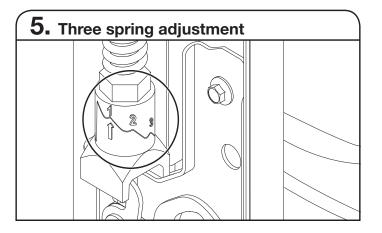
Each hinge has 3 different spring tension levels that it can be set to. The current tension level is indicated by an arrow. 1 is the lowest spring tension for light doors and 3 is the highest for heavier doors. 2 is the middle tension for door panel weights that fall between heavy and light.
