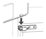
Fit the hinge **1** over the hinge lever latch **2** and slot it into place. Rotate the lever 3 clockwise and fasten the hinge.
