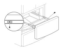
Insert the basket into the frame, and push the drawer back until it clicks into place.
