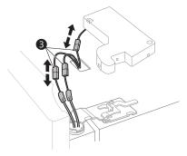
**3** Rotate the hinge lever **4** clockwise. Lift the top hinge **5** free of the hinge lever latch **6**.
