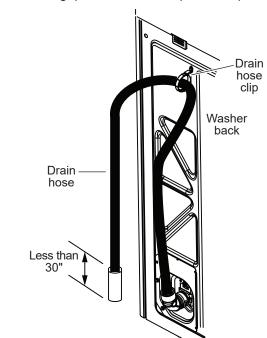
**NOTE:** Placing the drain hose too far down the drain pipe can cause a siphoning action. No more than 5" of hose should be in the drain pipe. There must be an air gap around the drain hose. A snug fit can also cause a siphoning action.
