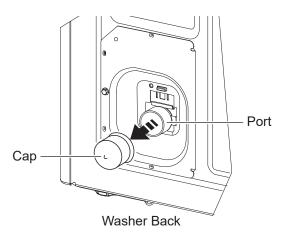
Connect drain hose to drain port on back of washer. Open clamp with pliers and slide onto hose end. Holding clamp open, push hose end onto drain port until fully seated. Release clamp between locating ribs on hose end. Outlet of hose end should be oriented vertically.
