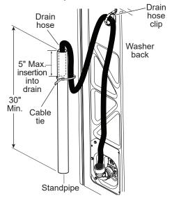
**NOTE:** Placing the drain hose too far down the drain pipe can cause a siphoning action. No more than 5" of hose should be in the drain pipe. There must be an air gap around the drain hose. A snug fit can also cause a siphoning action.
