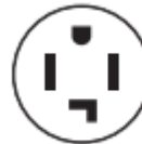
4-wire receptacle (14-30 R)
