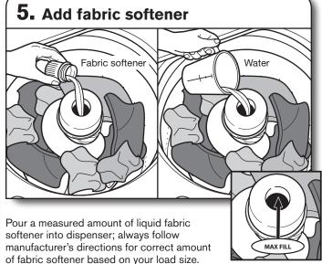
Dilute liquid fabric softener by filling the dispenser with warm water until liquid reaches the underside of the rim. See max fill line arrows.
