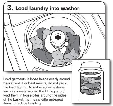
**IMPORTANT:** Do not tightly pack or force items into washer. Items need to move freely for best cleaning and to reduce wrinkling and tangling.
