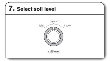
Once you select a cycle, select the soil level by turning the Soil Level knob to the desired setting.
