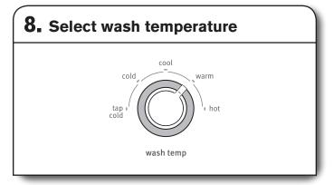
Once you select a cycle, select the wash temperature by turning the Wash Temp knob to the desired setting. Always read and follow fabric care label instructions to avoid damage to your items.
