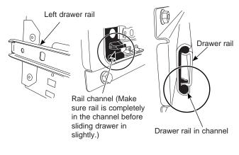
2. Place the right drawer rail inside the inner right rail guide channel at the top and slide it in slightly.
