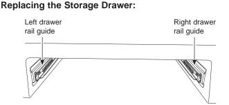
1. Rest the left drawer rail inside the inner left rail guide channel at the bottom and slide it in slightly.
