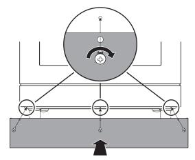
After the front skirting has been installed, the side skirting can be fastened correctly to the appliance. Use a screwdriver to remove the side screws.
