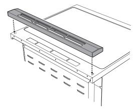
2. Make sure that you align the pins (**A**) of the backguard with the holes (**B**) on the cooktop.
