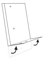
3. Place the template so that the thick vertical line drawn on it is aligned with the edge of the left side of the appliance.
