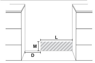
The grounded outlet should be located in the highlighted area in the image above. This area must have the following measures:
