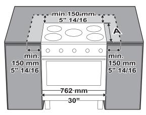
The side cabinet depth (clearance **A**) must match the front edge of the range side panel:
