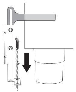
9. Push the cooker towards the wall, and at the same time, insert the bracket in the plate that is fastened to the rear of the appliance.
