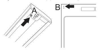
3. Secure the backguard to the top by the tightening the screws.
