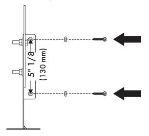
7. Use the following distances for the distance from the side of the appliance to the bracket holes.
