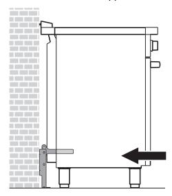
MARNING The rear vent trim has 3/16" (5 mm) standoffs to keep the appliance slightly away from the back wall. Do not remove or tamper with standoffs due to potential temperature issues.
