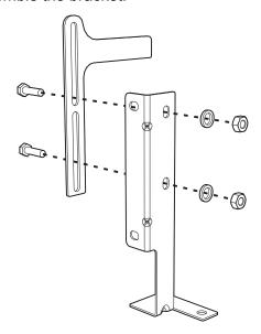
Align the base of the hook of the bracket with the base on the slot of the rear wall fastening bracket. Align the base of the fastening bracket with the floor and tighten the screws to fix the measurements.
