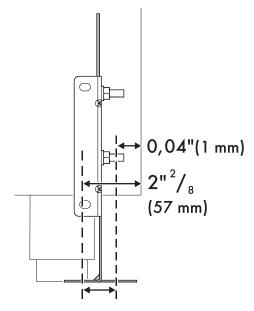
8. After having positioned and leveled the appliance, move the bracket close to the rear of the appliance and anchor it to the floor using the two washers and screws. A qualified technician must verify the suitability of the materials in accordance with the type and condition of the floor.
