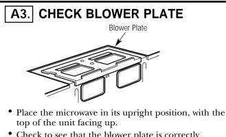
• Check to see that the blower plate is correctly installed on the unit.
