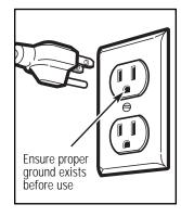
The power cord of this appliance is equipped with a three-prong (grounding) plug which mates with a standard three-prong (grounding) wall receptacle to minimize the possibility of electric shock hazard from this appliance. You should have the wall receptacle and circuit checked by a qualified electrician to make sure the receptacle is properly grounded.
