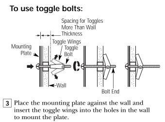
**NOTE:** Before tightening toggle bolts and wood screw, make sure the bottom of the mounting plate touch the bottom of the cabinet when pushed flush against the wall and that the plate is properly centered under the cabinet.
