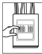
CAUTION: For personal safety, remove house fuse or open circuit breaker before beginning installation to avoid severe or fatal shock injury.
