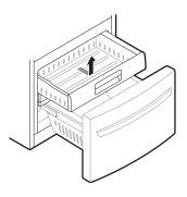
4 Remove the Durabase basket from the rails. Remove the screws from the rails at both ends.
