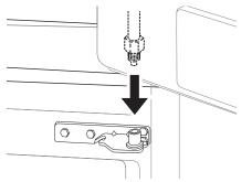
2 Fit the hinge ① over the hinge lever latch ② and slot it into place. Rotate the lever ③ counterclockwise to secure the hinge.
