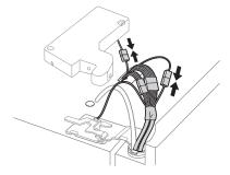
**4** Push the water supply tube into the hole on the top case and pull it through the backplate.
