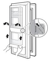
2 To replace the case, line up the tabs on the case with the slots on the door and push down until it snaps into place.
