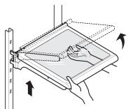
**3** To assemble, tilt the front of the shelf up and guide the shelf hooks into the slots at a desired height.
