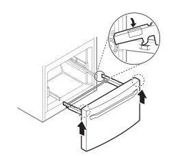
**3** Lower the door into its final position and insert the screws in the rails on both sides.
