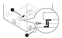
3 Preassemble a 4" (10 cm) elbow 5 to the next 4" (10 cm) duct section, and secure all joints with duct tape. Be sure that the male end of the elbow faces AWAY from the dryer. Insert the elbow/duct assembly through the side opening and press it onto the adapter duct. Secure it in place with duct tape. Be sure that the male end of the duct protrudes 1 1/2" (3.8 cm) to connect the remaining ductwork. Attach the cover plate 6 to the back of the dryer with the included screw.
