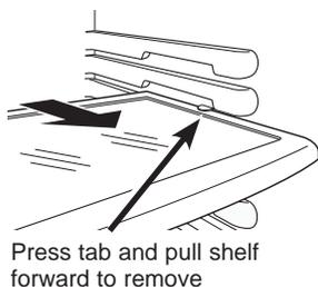
**To replace or relocate:** Line the shelf up with the supports and slide it into place. The shelf can be repositioned when the door is at 90° or more. To reposition the shelf, slide the shelf past the stops and angle downward. Slide shelf down to the desired position, line up with the supports and slide into place. Make sure you push the shelves all the way back in before you close the door.
