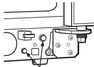
Turn the front roller adjusting screws **clockwise to raise** the refrigerator, **counterclockwise to lower** it. Use a 3/8" hex wrench with extension, or an adjustable wrench.
