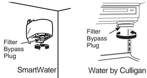
To use the filter bypass plug on Water by Culligan™ models, you must first remove the filter adapter from the cartridge holder by turning it to the left.
