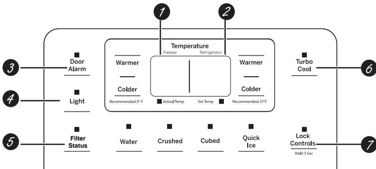
The temperature controls are preset in the factory at **37°F (2.8°C)** for the refrigerator compartment and **0°F (-17.8°C)** for the freezer compartment. Allow 24 hours for the temperature to stabilize to the preset recommended settings.
