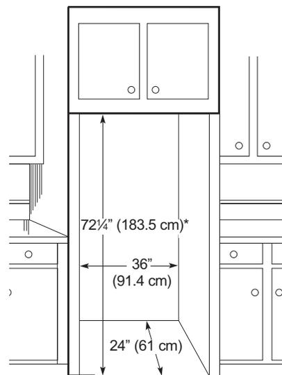
\*72-1/4" (183.5 cm) required for full adjustment of mobility wheels. If cabinets installed above refrigerator have doors that are flush to the top of the opening for the refrigerator, then an additional 1/8" may be required to provide clearance for cabinet doors to open freely.
