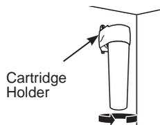
5. Slowly turn it to the right until the filter cartridge stops. **DO NOT OVERTIGHTEN.** As you turn the cartridge, it will automatically raise itself into position. The cartridge will move about 1/2 turn.
