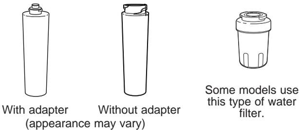
2. On models without a replacement indicator light, apply the month and year sticker to the new cartridge to remind you to replace the filter in six months.
