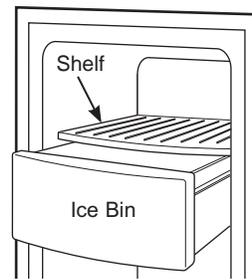
To reach the power switch, pull the shelf straight out. Always be sure to replace the shelf.
