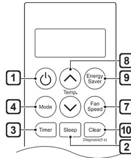
**Energy Saver** - In this mode the compressor and fan turn off when the set temperature is achieved. Approximately every 3 minutes the fan turns on to allow the unit sensor to accurately determine if more cooling is needed.
