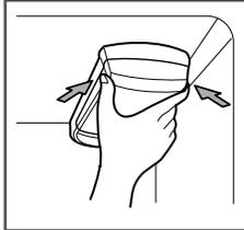
**NOTE:** Replacing the water filter causes a small amount of water (around 1 oz. or 25 cc) to drain. Place a cup under the front end of the water filter cover to collect any leaking water. Hold the water filter upright, once it is removed, to prevent any remaining water from spilling out of the water filter.
