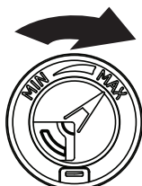
Clockwise to reduce water drops and hard water spots
