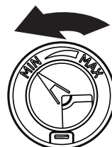
Counterclockwise to reduce foaming
