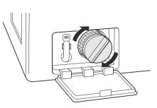
**8** Close the drain pump filter cover.
