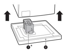
2 Remove the bolt assemblies.
