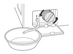
**5** Clean the pump filter and opening.
