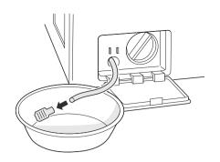
**4** Remove the pump filter.
