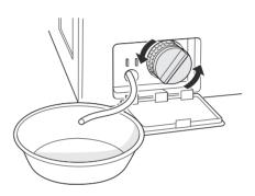
**5** Clean the pump filter and opening.
