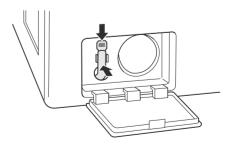
**7** Insert the drain pump filter.
