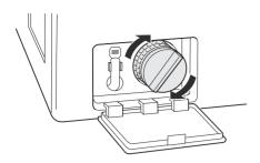
Close the drain pump filter cover.
