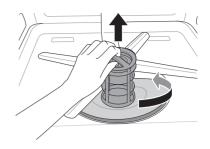
Clean the filters with a soft brush under running water. Reassemble the filters before reinstalling them.
