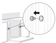
**2** Drive a wood screw through the mounting bracket and into the cabinet frame.
