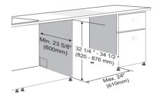
2 To allow for proper clearance of plumbing and electrical, use the template included with the literature to determine the clearance on the side of the cabinet where the cabinet meets the back wall. Using a 2 1/2" diameter hole saw, drill a hole in the target area as shown on the template.
