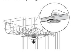
Remove food particles by rinsing or shaking the spray arm.
