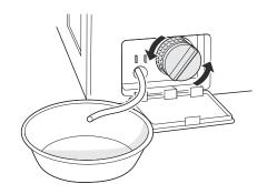
Clean the pump filter and opening.
