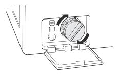
Close the drain pump filter cover.
