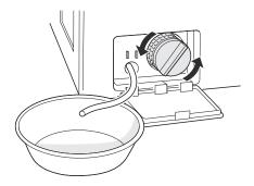
**5** Clean the pump filter and opening.
