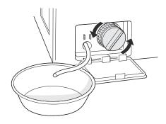
**5** Clean the pump filter and opening.
