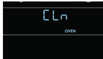
Figure 31: Clean lock icon blinks as door unlocks
