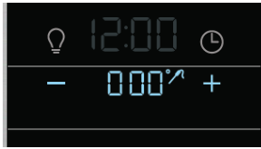
Figure 18: Probe inserted and ready to set temperature
