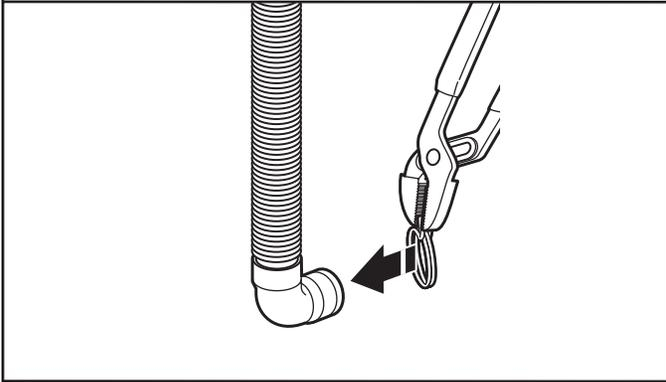
If clamp is not already in place on elbow end of drain hose, slide it over end as shown. Squeeze clamp with pliers and slide black elbow end of drain hose onto black drain port and secure with clamp.
