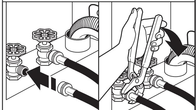
Verify location of hot and cold faucets. Attach hose to hot water faucet. Screw on coupling by hand until it is seated on washer. Use pliers to tighten couplings an additional two-thirds turn. Repeat this step with second hose for cold water faucet.
