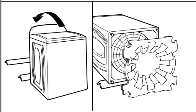
To avoid damaging floor, place cardboard supports from shipping carton on floor behind washer. Tip washer back and place on cardboard supports. Remove shipping base by rotating base 90° to the right. Set washer upright.
