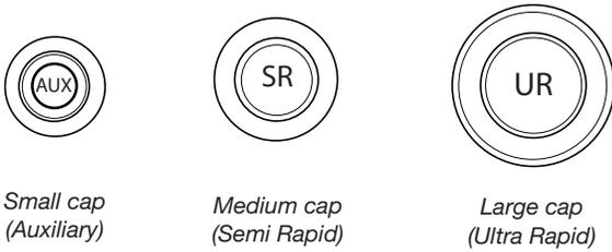
Burner caps should be level when properly positioned. If burner caps are not properly positioned, surface burners will not light. The burner cap should not rock or wobble when properly aligned.
