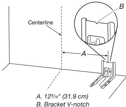
4. Drill two  $\frac{1}{8}$ " (3 mm) holes that correspond to the bracket holes of the determined mounting method. See the following illustrations.
