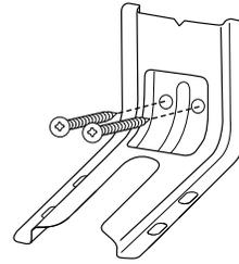
5. Using the Phillips-head screws provided, mount anti-tip bracket to the wall or floor with #12 x  $1\frac{5}{8}$ " (4.1 cm) screws provided.
